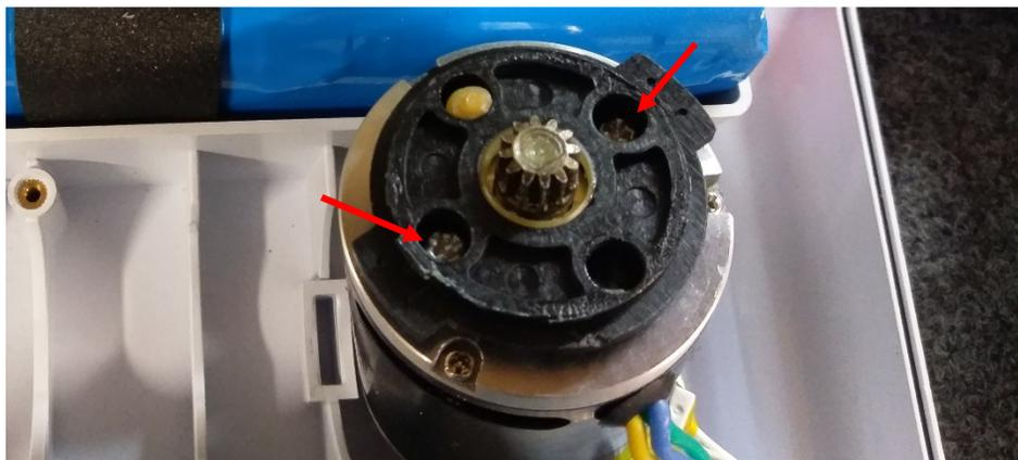
**5-Remove the base connector from the new gearbox by rotating. In this case it is white in color. Use caution that the gears are not disturbed. Now Attach it to the motor end.**
