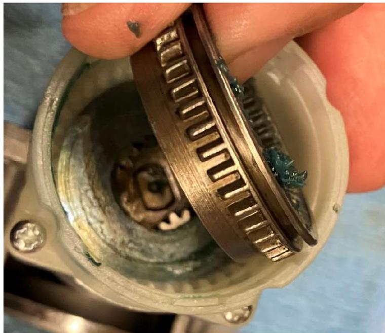
**STAGE-5 INSTALL GEAR TRANSFER**
