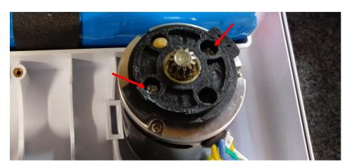
5-Remove the base connector from the new gearbox by rotating. In this case it is white in color. Use caution that the gears are not disturbed. Now Attach it to the motor end.
