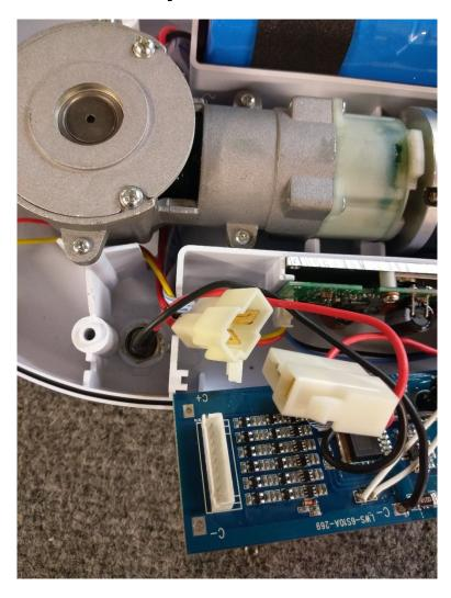
3-Locate outer prong and unused center short prong on the PSR component.
